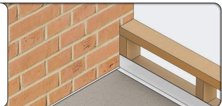
\*PLEASE NOTE: Voids larger than 20mm must to be filled with structural material and sealed correctly prior to balcony panel installation.
